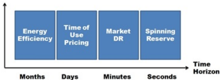
Figure 2: Different time horizon in DSM, based upon [1]
