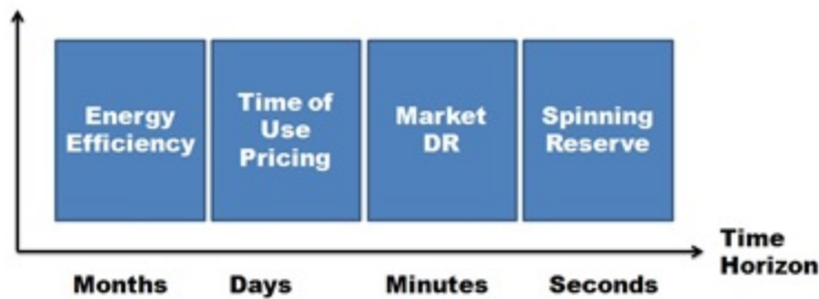
Figure 2: Different time horizon in DSM, based upon [1]
